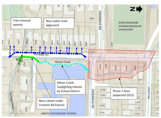
In addition to improving fish habitat in Kilmer Creek, this work will reduce the likelihood and severity of flooding events in the future. The new culvert will enable fish to pass through and will be able to convey a 200-year flood event that takes into account the anticipated impacts of climate change.
